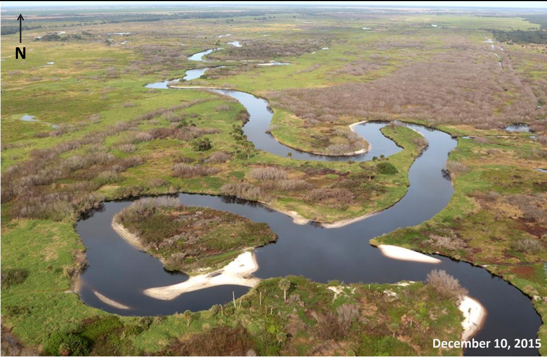
Micco breakthrough under lower discharge exposes sand deposits resulting from both the former and new routes that flow has taken. A sandbar has formed across the entire length of the abandoned channel (Discharge at s65A was ~300cfs).
