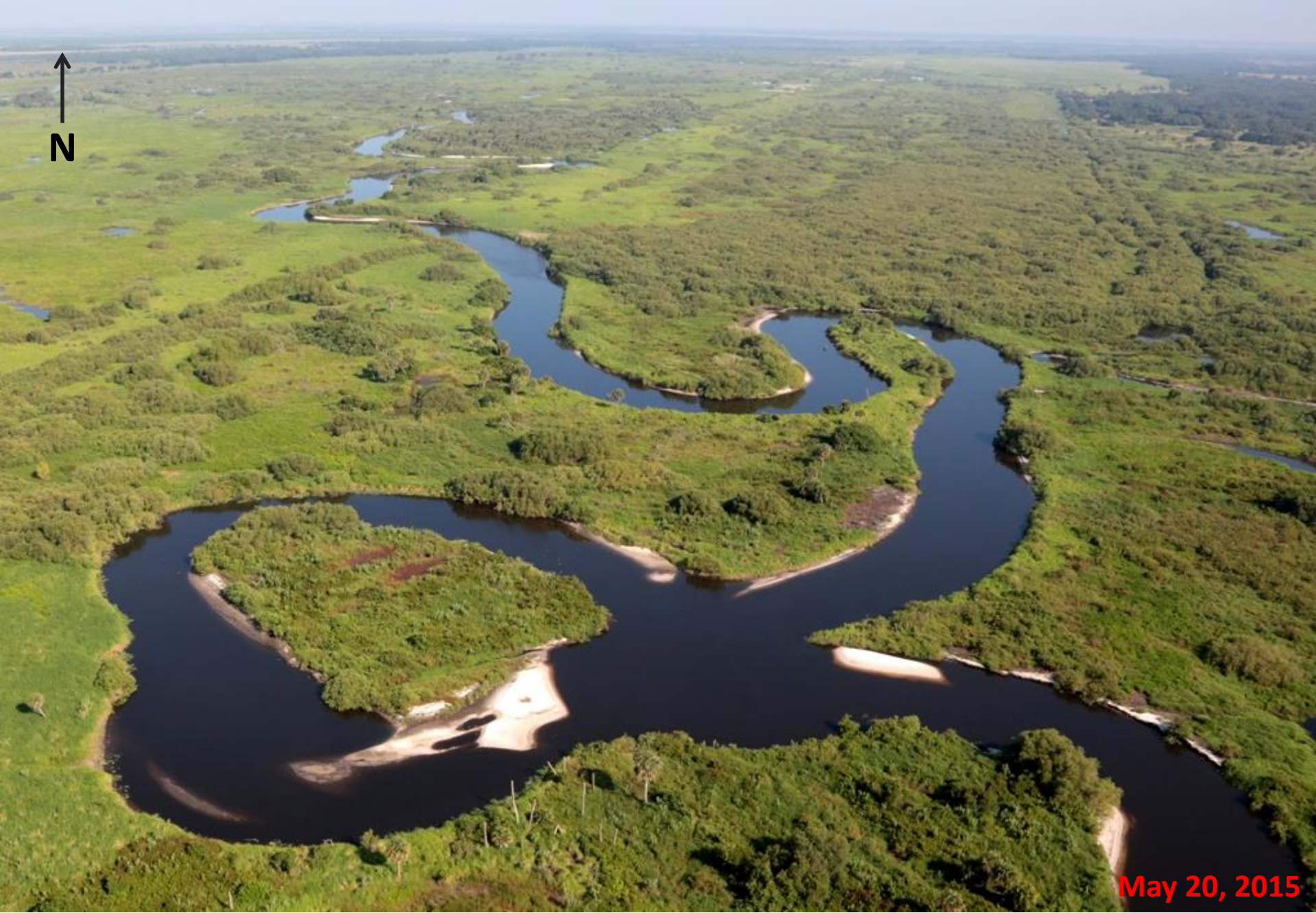
Micco breakthrough under lower discharge exposes sand deposits resulting from both the former and new routes that flow has taken. (Discharge was ~300 cfs at s65A since May 8).
