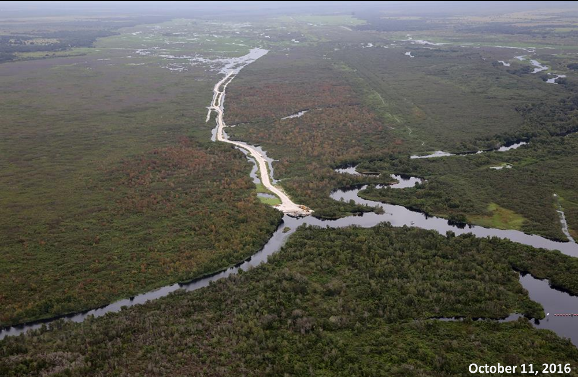
Looking north up the MacArthur Ditch backfill project. The contractors are done hauling spoil, and are temporarily on hold until the water levels recede below final grade height before they can level the haul road.
