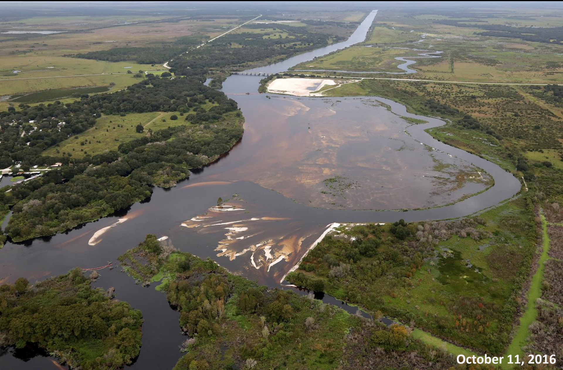
Looking north at the north section of the Reach 3 backfill, which was completed by the end of August and shortly after was inundated with high flows.
