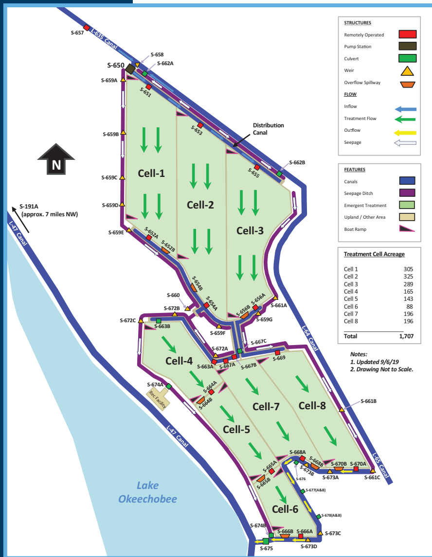
Structures and features map for LRSTA Phase I and II. Note: The remotely operated structures are each constructed of four weir gates and one box culvert.
