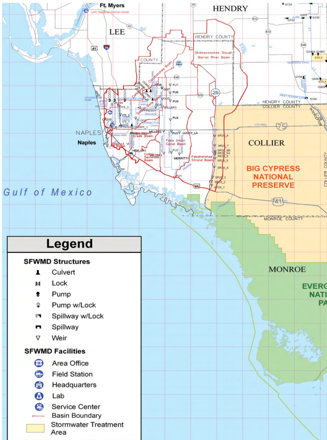
Figure C-10. Major drainage basins and water management features within the Big Cypress Basin.
