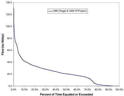
Dry Sesaon Volume Probability Curve (Nov 1- May 31) 160.0 -MIN (Target & 2000 W\Project) 140.0 120.0 100.0 Flow (ac-ft/day) 80.0 60.0 40.0 20.0 0.0% 60.0% 70.0% 80.0% 90.0% 100.0% 10.0% 20.0% 30.0% 40.0% 50.0% Percent of Time Equaled or Exceeded
