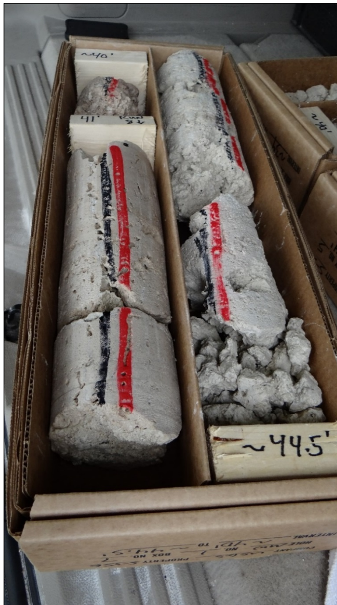
Figure 3. A typical field photograph of a core sample obtained from the pilot hole.
