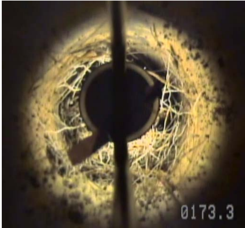
Figure 17. Tubular mineral growth crisscrossing the borehole below the base of the casing during downhole video logging of OSF-52 in February 2018.
