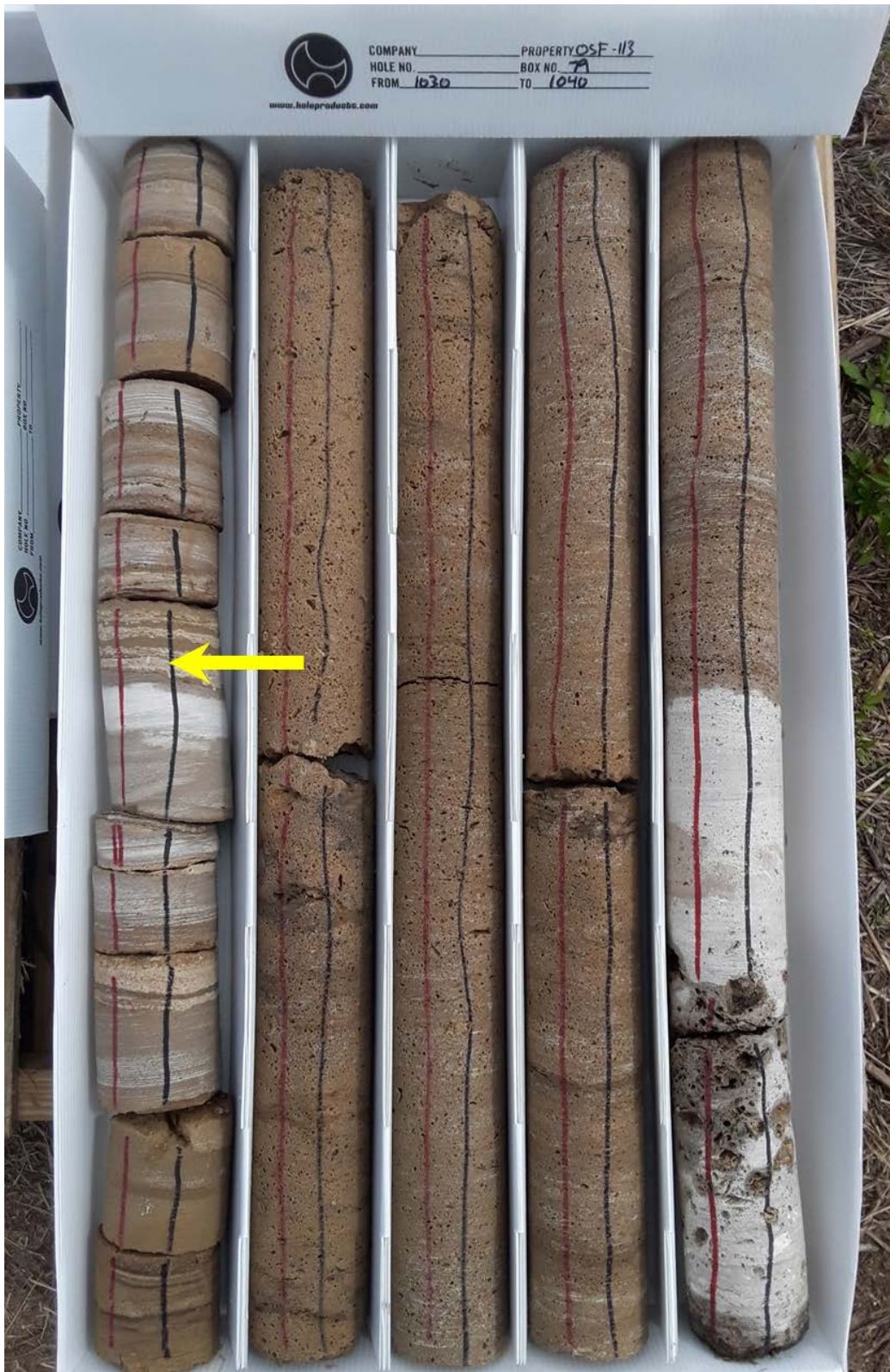
Figure 4. Core interval (1,030 to 1,040 ft bls) containing celestine at OSF-113. Arrow marks sampled depth.
