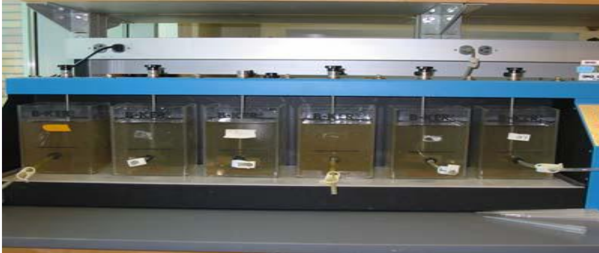
Figure 3-1 Phipps and Bird PB-700 jar test system
