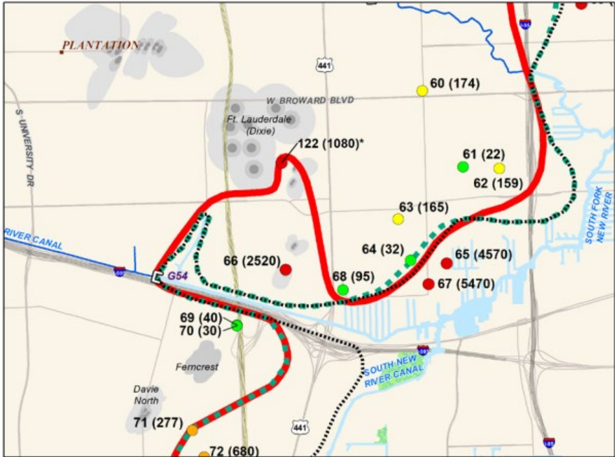
Figure D-17. Changes in the saltwater interface position around the Fort Lauderdale Peele-Dixie wellfield.
