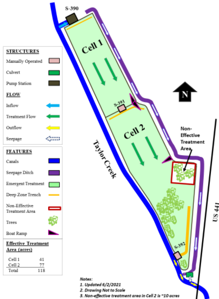
Figure 7-2. Taylor Creek STA structures, flows, and features.
