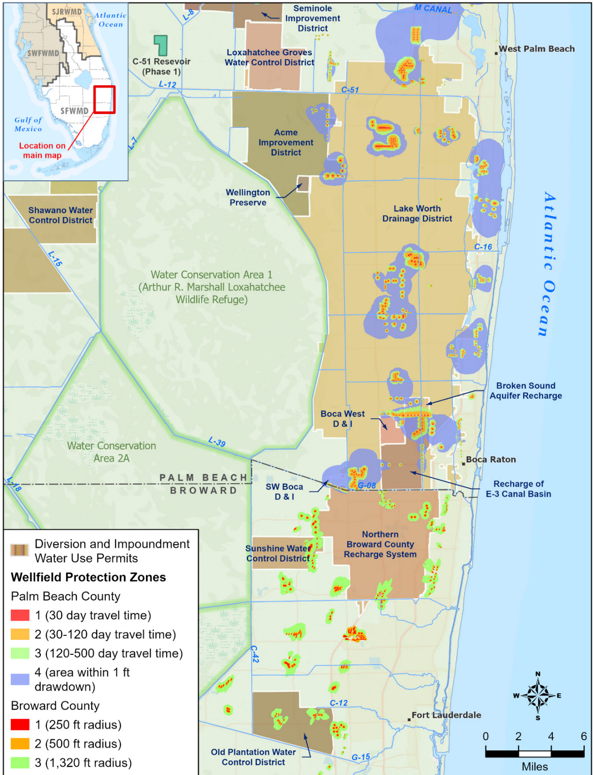
Figure 5-4. Water control districts that divert regional water to recharge Public Supply wellfields in the LEC Planning Area.
