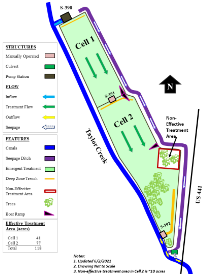
Figure 7-2. Taylor Creek STA structures, flows, and features.
