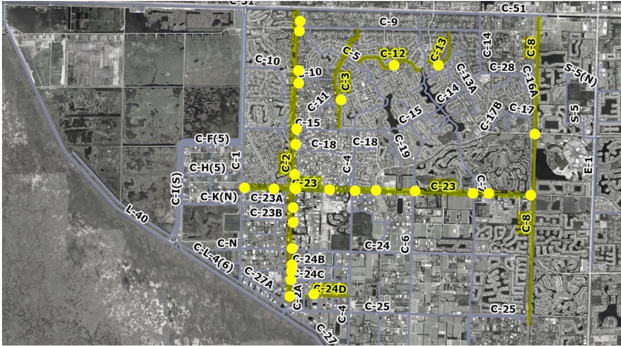
Figure 16. This graphic from the Acme video shows the dense network of canals that have been created to allow development in this former wetland known as Wellington to take place. The yellow markers indicate many culvert upgrades that have already gone into the upgraded system. The video also notes other upgrades that will be applied to the drainage system, such as the “Pumpstation 2 Rehabilitation Project,” which is currently in the planning stage. That project would rehabilitate an older, currently unused pumpstation on the border of the Loxahatchee National Wildlife Refuge to once again pump water south into the refuge in anticipation of major flooding that could overwhelm Wellington’s canal system and other infrastructure.
