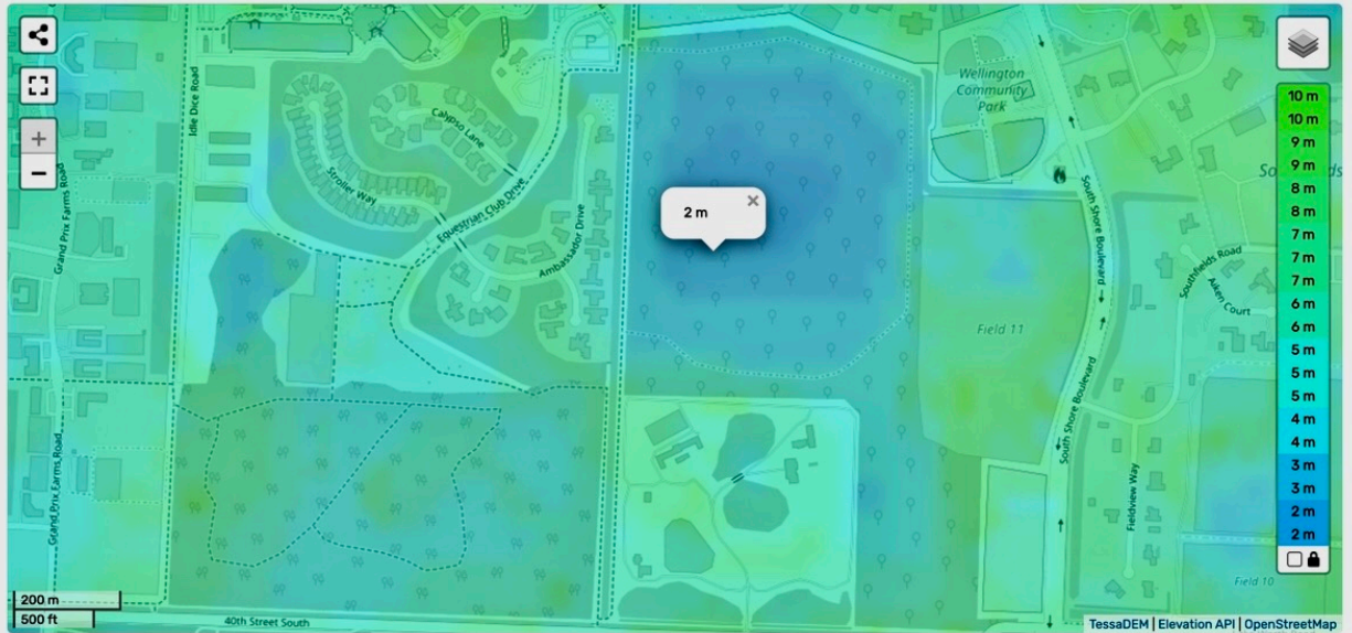
Figure 12. Zoomed version of the topographic elevation map shows the elevation of Wellington South (Parcel B) is as low as two meters (about 6.5 feet) above sea level. The elevations seen in the numerous developments immediately to the north, northwest, and west of Wellington South generally show up on the elevation map set as 6 to 8 meters (19-26 feet). In its current undeveloped state (without the fill that would be necessary to develop this site), Wellington South is very likely providing significant drainage and natural flood management to the residential areas as well as the horse farms that surround it.
