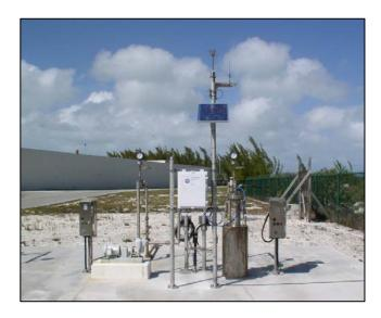
Figure 3-3 -- A continuous groundwater monitoring station at an FAS well.
