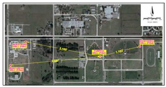
Figure 3-11 -- Well configurations during the Clewiston APT.
