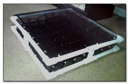
Figure 8-1 -- Cages for freshwater mussel exposures.
