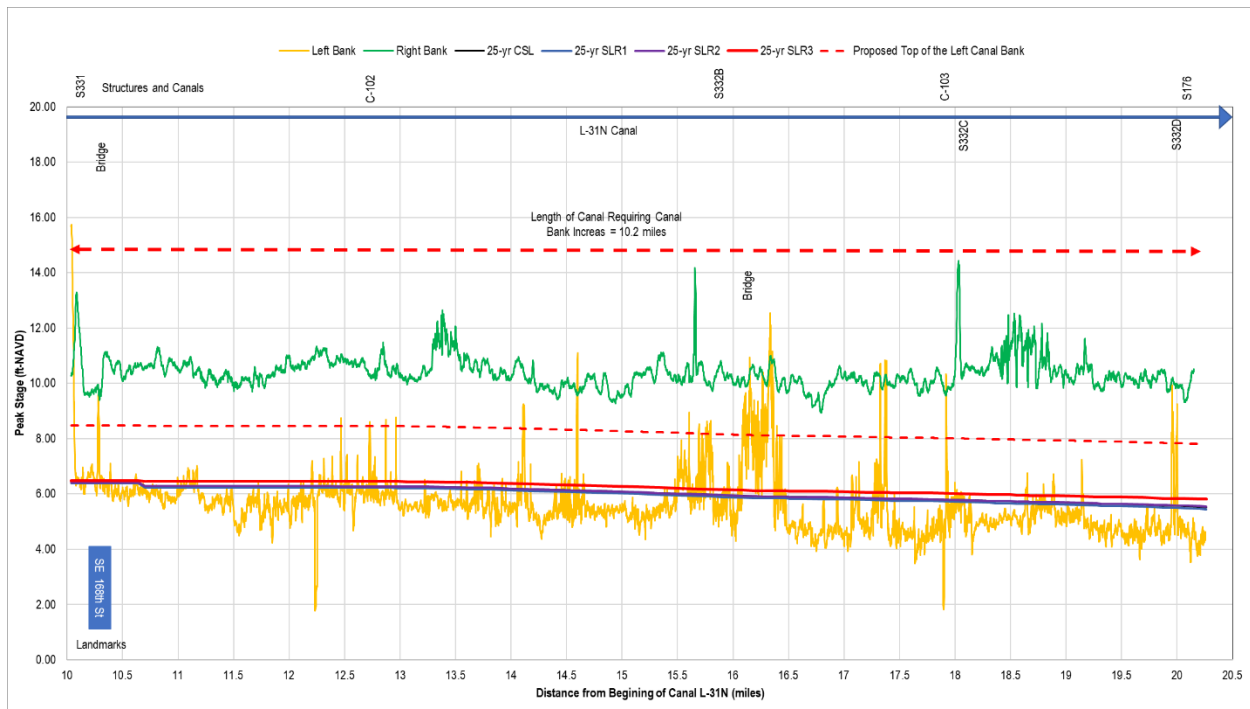
Figure 83. Profile of Peak Stages in Canal L-31N from Pump Station S331 to Structure S176 for 25-yr Design Event and Proposed Top of Left Canal Bank Elevation. Data from the Flood Protection LOS Performance Metric PM1 of the C-111 FPLOS
