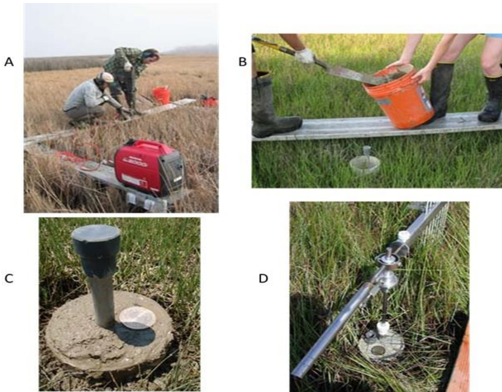
A. Driving rods after constructing the platform. B. Cementing collar and receiver. C. View of a completed receiver with a brass marker. D. SET arm attached to receiver for first readings. Pictures from: http://www.pwrc.usgs.gov/set/
