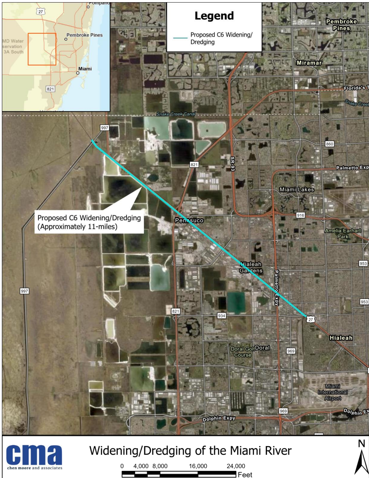
Figure 30: Proposed location of widening/dredging the Miami River.
