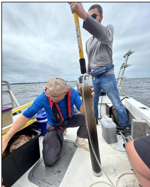
Figure 1. Sediment core photograph. Cores were collected from LOCB using a 3.5" diameter telescopic pole corer.
