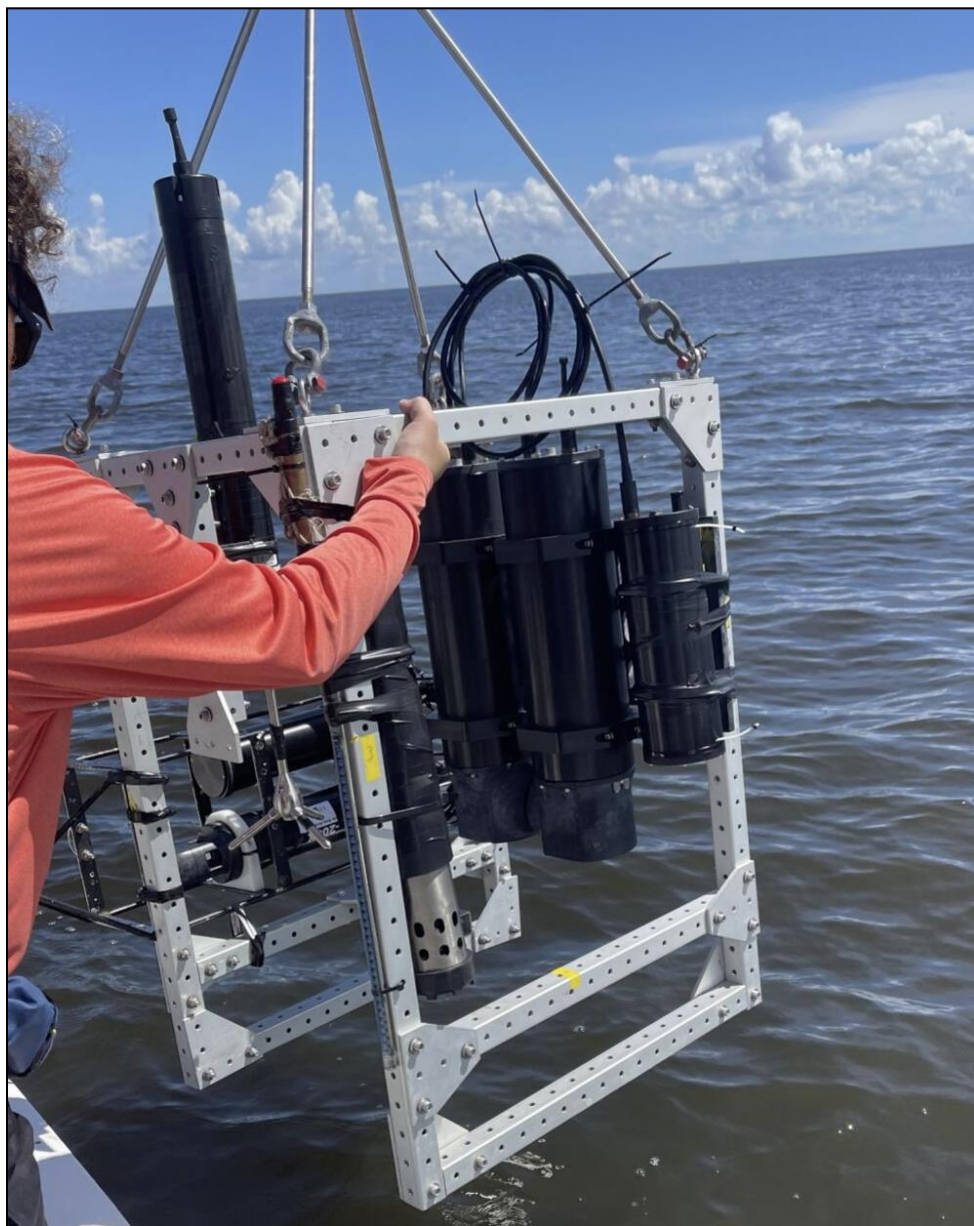
Figure 1. Benthic lander platform. Photo of the system illustrating the position of the sonde, AUTOHOLO, and LISST-200X.
