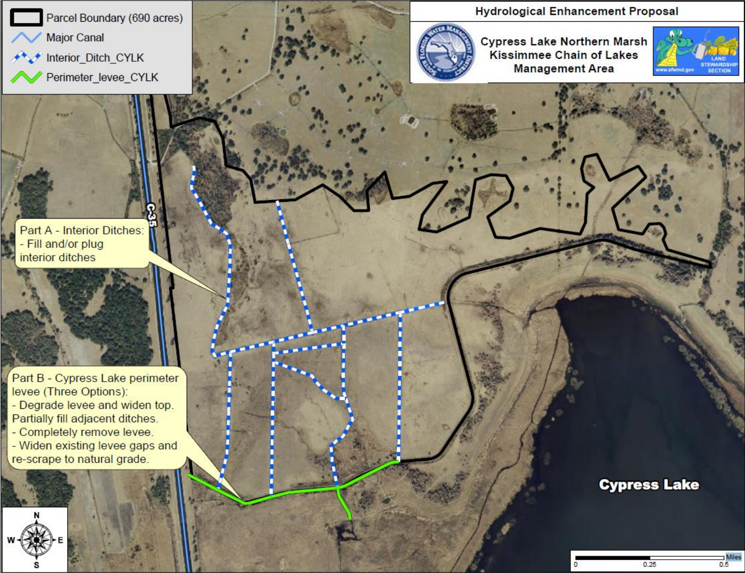
Figure 14. Proposed additional hydrological restorations within Cypress Lake.
