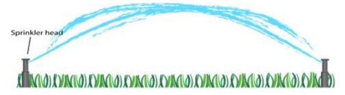
Area between heads is receiving the same amount of water. In accordance with Appendix F of the Plumbing Volume of the Florida Building Code, sprinklers should be adjusted and spaced to avoid watering impervious surfaces such as sidewalks, buildings and roadways.
