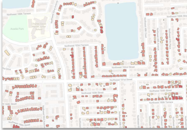
Figure 19 Example shapefile output for a scenario run with the SFWMD-FIAT (legend omitted for privacy). Each object can be clicked to obtain a wealth of exposure data information and damage assessment results.
