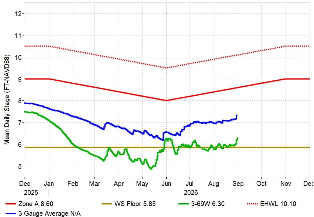
Figure EV-3. WCA-3A stage hydrographs (three-gauge average, 3-69W) and regulation schedule.
