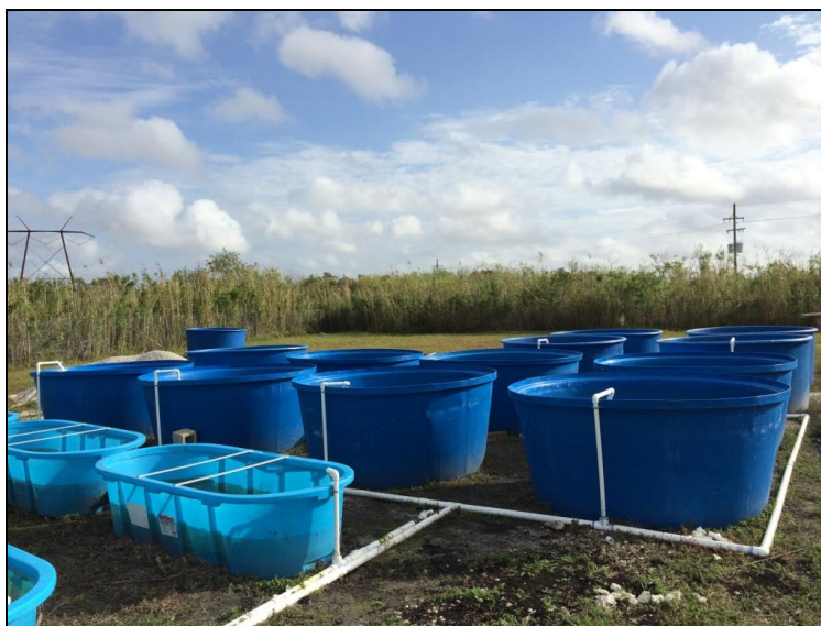
Figure 1. Mesocosms were established at a range of water depths to explore the effects of operating conditions on P removal effectiveness and biological community response. The shorter tanks (to the lower left) were plumbed 4 in-series at water depths of 23 or 46 cm. The larger mesocosms were plumbed 2 in-series and were also established at 46 cm, before transitioning to 69 cm or 92 cm water depths.
