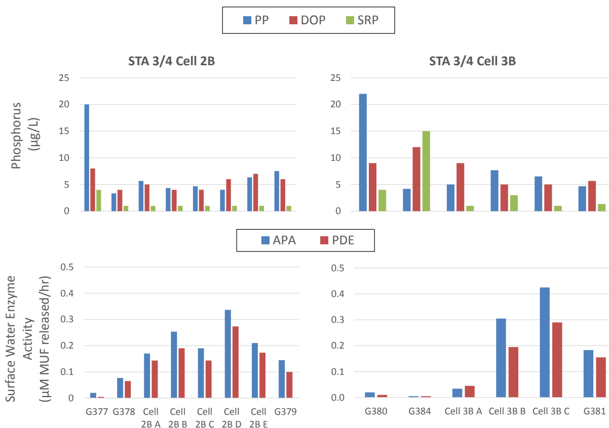
Figure 14. Phosphorus concentrations and phosphatase enzyme activities in two “back-end” cells of STA-3/4 on July 28, 2015.
