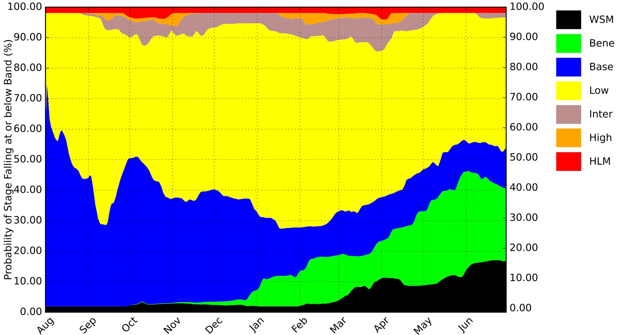
The width for each band gives the probability of stage falling in that band, as defined by the operational schedules
